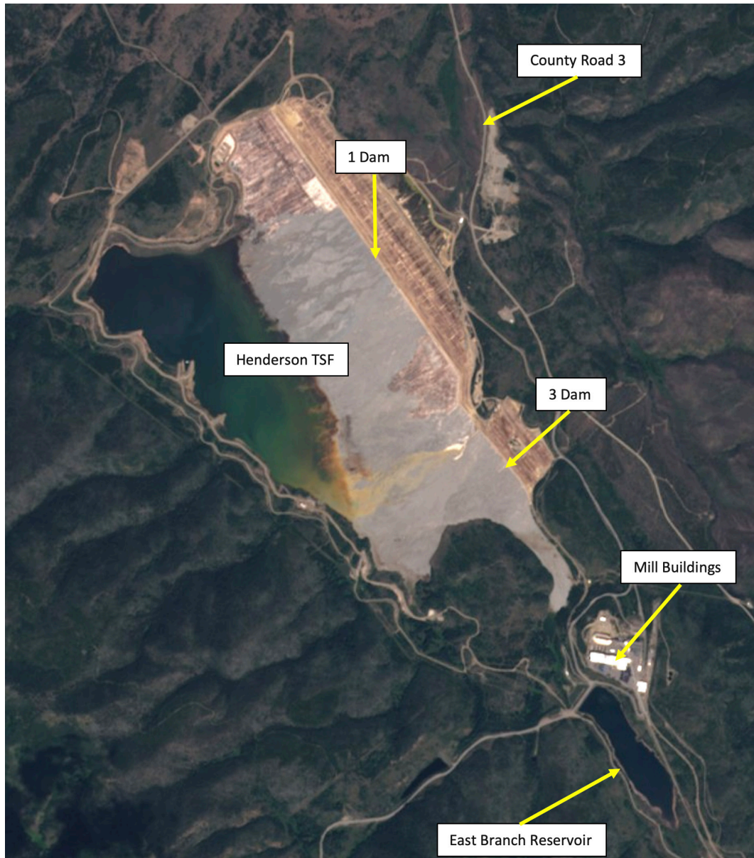
Figure 3. General Henderson Mill Layout (August 29, 2023).
